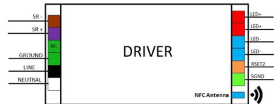
Both output positive and negative connectors are equivalent (same electrical point).
